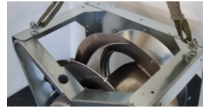
Fitting lifting lugs in the positions provided
